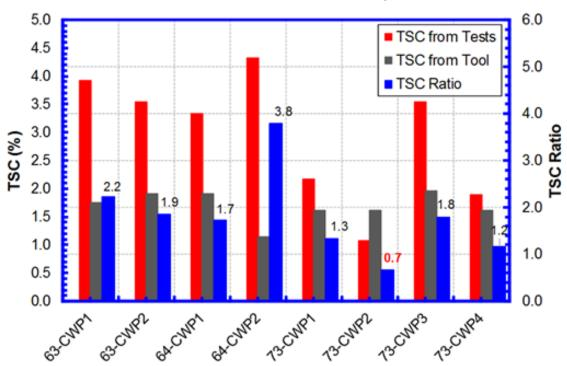
Figure E-9 Comparison of measured TSC from curved wide plate (CWP) tests of vintage girth welds and predicted TSC from the PRCI SIA-1-7 tool [27]. Specimen 73-CWP2 had a large preexisting flaw that was not identified prior to the test. This flaw led to the unexpected low TSC.
