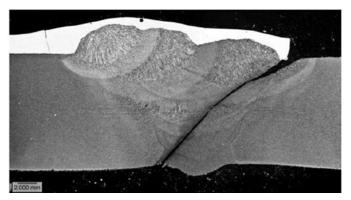
Figure E-4 Failure of a girth weld with weld strength undermatching in the absence of weld flaws
