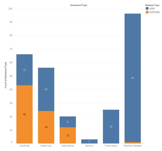
Figure A-1 Incidents by hazards type and leak vs. rupture (over a 20.5-year period)
