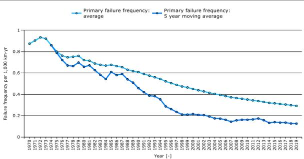
Figure A-11 EGIG primary failure frequency [2]
