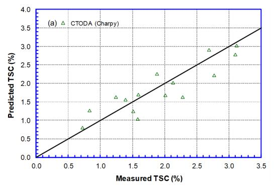
Figure E-8 TSC predicted by the Level 2 procedure of PRCI-CRES tensile strain model vs. TSC measured from full-scale tests of mechanized girth welds [26]
