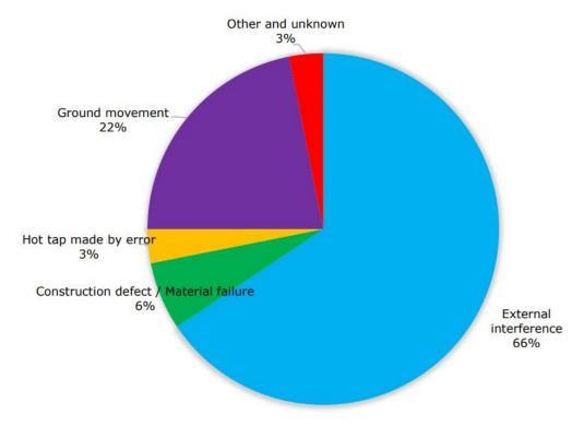
Figure A-14 EGIG distribution of incidents with hole leak size from 2010-2019 [2]
