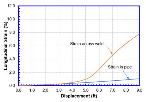
Figure E-6 Comparison of strain across a girth weld and strain in the pipe body in a weld joint with weld strength undermatching
