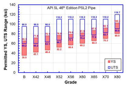
Figure D-2 Permitted ranges of yield strength and UTS for PSL2 pipes in API 5L
