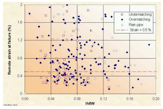
Figure E-7 Remote strain measured at failure of curved-wide plate (CWP) test specimens with planar flaws with height *h* and length *l*. The CWP has an overall gauge width of *W* and wall thickness of *t*. (a) full range of strain, (b) strain range up to 2.0%.
