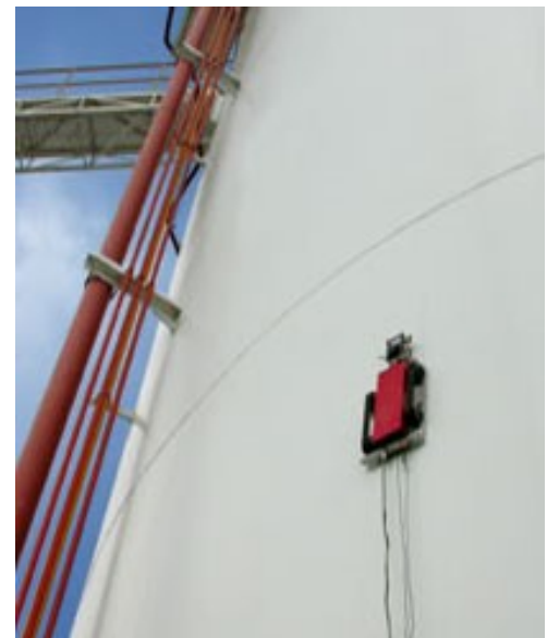
Tank Roof & Wall UT Scanners
