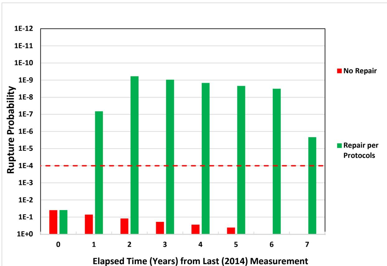
Figure 6. POF and SF for Class 3 Section as a Function of Time for SCC Anomalies – Both PHMSA and INGAA Protocols lead to the same outcomes and hence there is no distinction in the graphs
