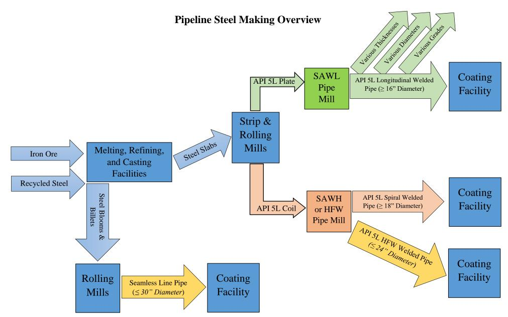
**Figure 1**: The flow diagram above represents a high-level overview of the manufacturing process for pipeline-quality steel and line pipe. For each welding method and seamless line pipe, a range of thicknesses, diameters and grades are available – this is shown for SAWL pipe as an example. Diameter ranges are approximate and may not represent every manufacturer.
