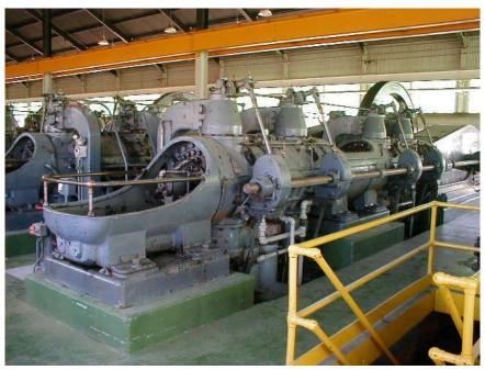
Figure 4-1. Horizontal Engine
