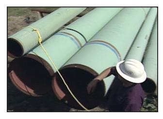
around the world manufacture API 5L line pipe for the natural gas industry. Pipe mills produce two types of line pipe: seamless and welded.
