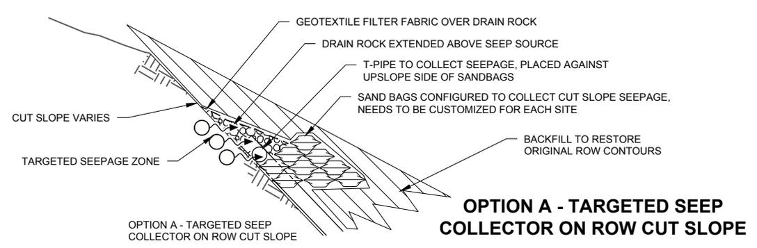
**OPTION A - TARGETED SEEP COLLECTOR ON ROW CUT SLOPE**
