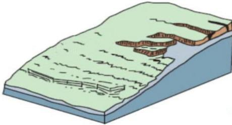
**Figure 2-14: Example Slope Soil Creep (USGS 2004)**
