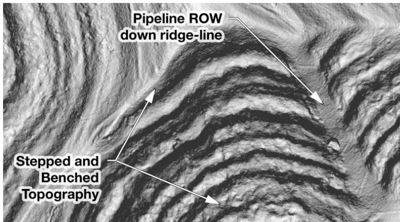
**Figure 2-2: LiDAR hillshade example of stepped and benched topography in northern West Virginia [Notes: (1) Pipeline ROW following ridge down slope; (2) See discussion of LiDAR in Section 2.4; (3) Disturbed terrain along and below the benches describes landslide movement] (Williams 2015)**
