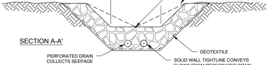
MIN. 3 FT WIDTH VARIES DEPENDS ON REQUIRED FLOW, MAY BE V-SHAPED (SEE DASHED) FOR LOW FLOW CONDITIONS
