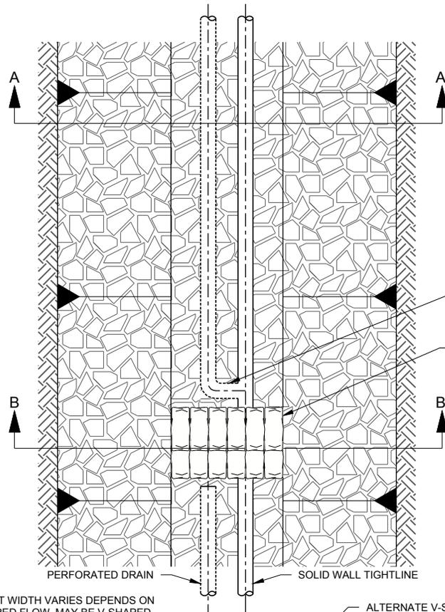
MIN. 3 FT WIDTH VARIES DEPENDS ON REQUIRED FLOW, MAY BE V-SHAPED (SEE DASHED) FOR LOW FLOW CONDITIONS
