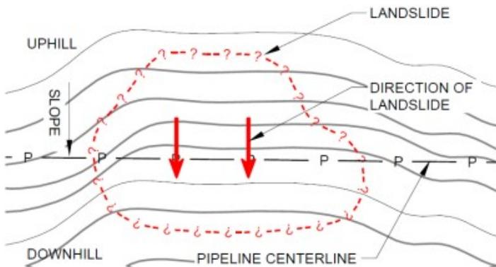
Figure 3-9: Conceptual Schematic for Sidehill Landslide (Williams 2015)
