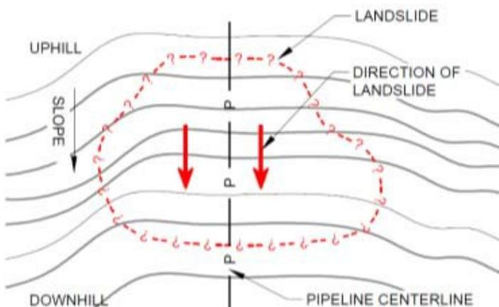
Figure 3-10: Conceptual Schematic for Planar Landslide (Williams 2015)
