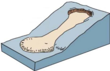
**Figure 2-13: Example Earth or Debris Flow (USGS 2004)**
