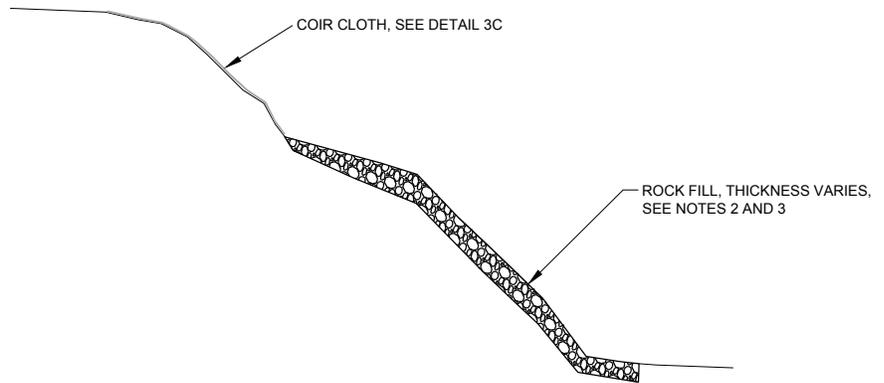
**A** **ROCK ARMORING ON DISTURBED SLOPE**
