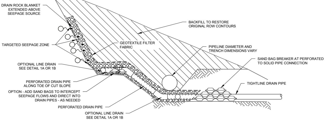
**OPTION B - TARGETED SEEP COLLECTOR ON ROW CUT SLOPE**
