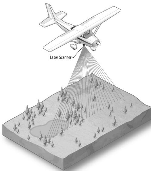
**Figure 2-4: Airborne LiDAR data collection system schematic (Williams 2015)**
