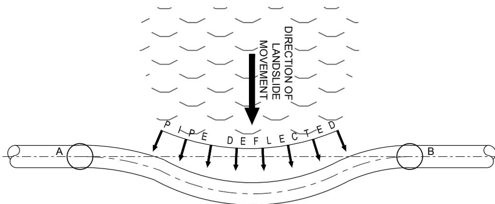
DURING STRAIN RELIEF EXCAVATION
