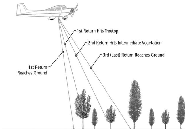
**Figure 2-5: Multiple Returns from LiDAR Laser Pulses (Williams 2015)**
