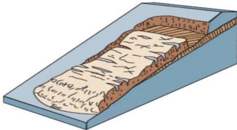
**Figure 2-12: Example Shallow Translational Landslide (USGS 2004)**
