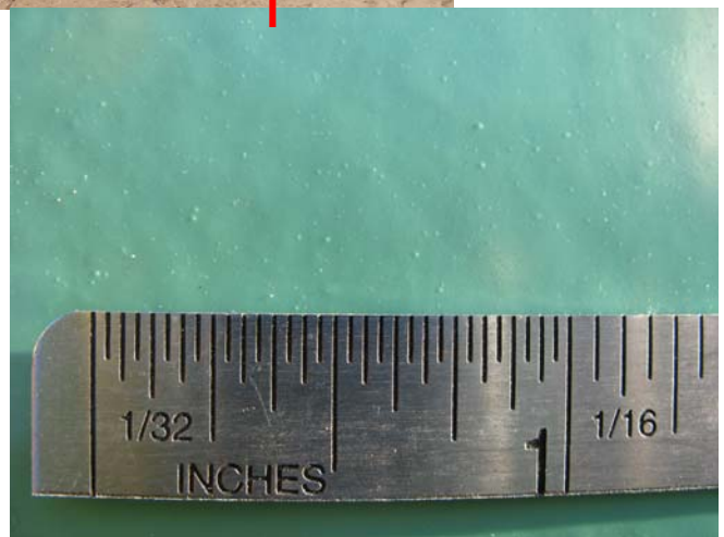
The above images of the micro-cracks observed on the coating pipe body illustrated by the red and yellow markers. The micro-cracks extended approximately 40ft. upstream and downstream of the rupture site, after which undamaged pipe coating was visually observed.
