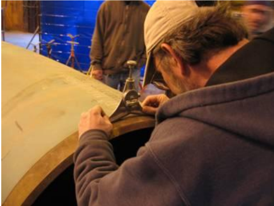
Figure 23. Center finder being used to locate TDC
