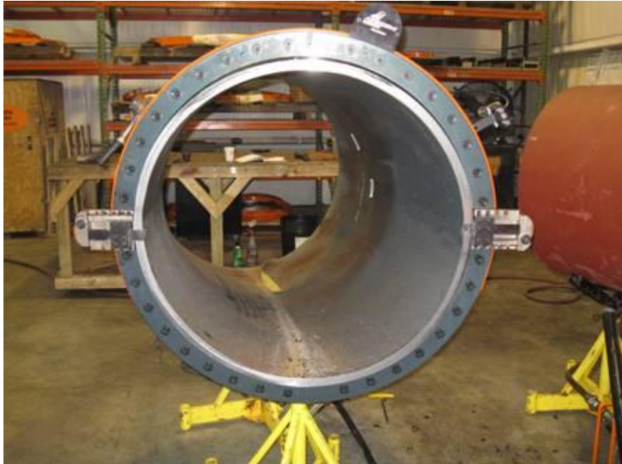
Figure 49. Steel Split Frame® equipment with cutting blade attachments mounted on 36 inch by 0.500 inch thick induction bend
