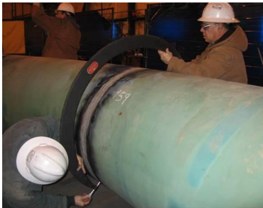
Figure 29. OD measurement using micrometer
