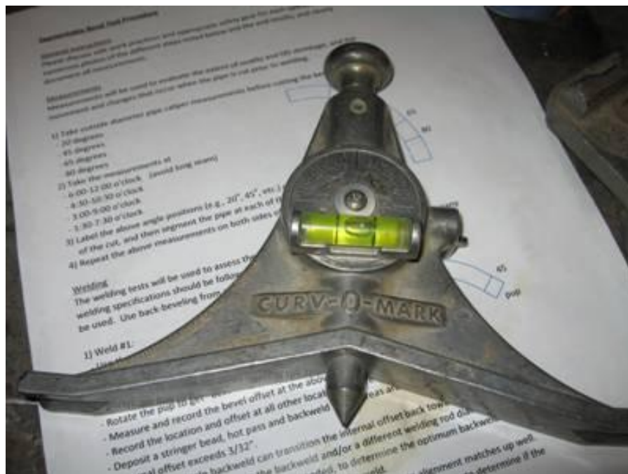
Figure 22. Center finder for locating top-dead-center, intrados, and extrados
