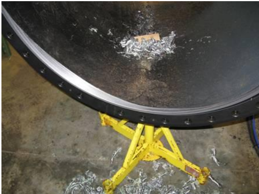
Figure 54. Completed internal taper
