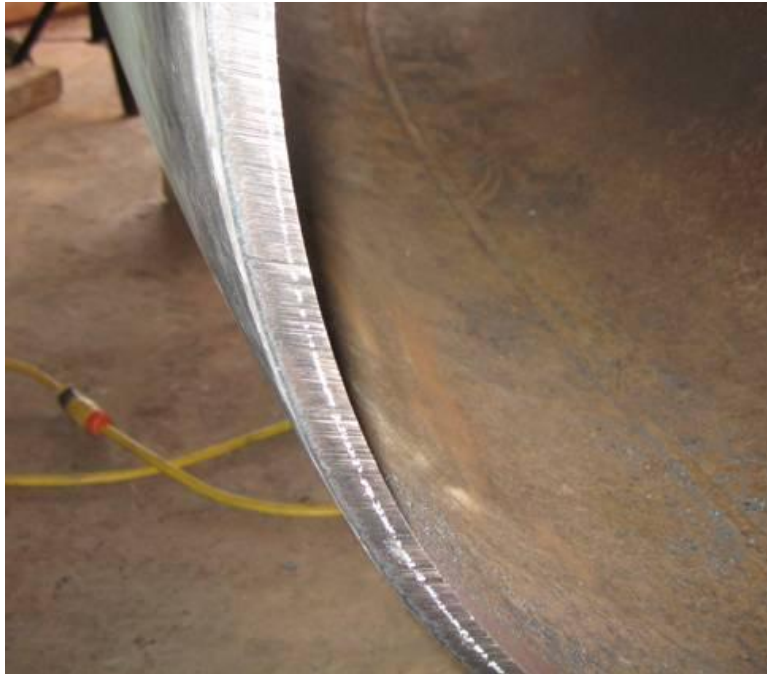
Figure 36. ID of pipe pup section marked on bevel of segmented bend with soapstone
