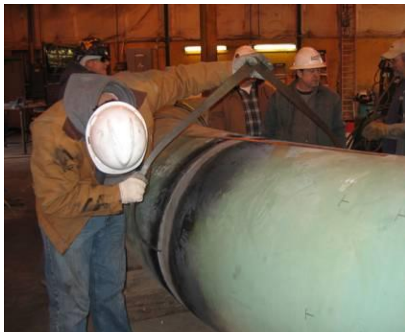
Figure 27. OD measurement using calipers – Part 1
