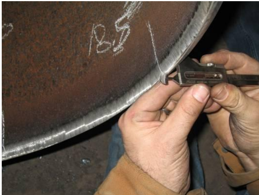
Figure 41. Measurement of wall thickness at weld bevel after transitioning
