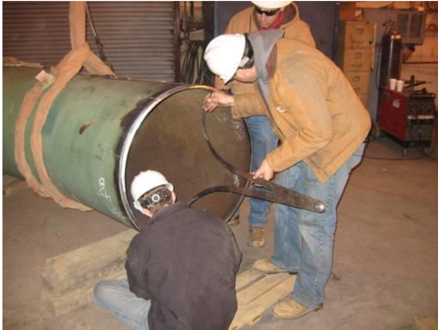
Figure 31. ID measurement using calipers
