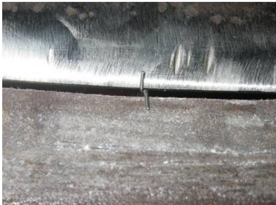
Figure 44. Measurement of high-low misalignment – Part 2
