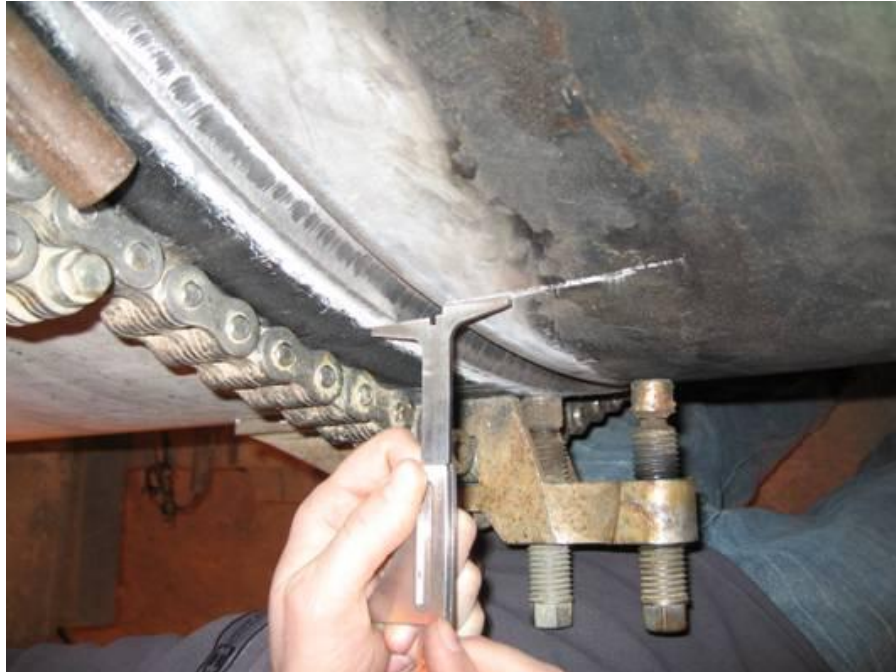
Figure 43. Measurement of high-low misalignment – Part 1
