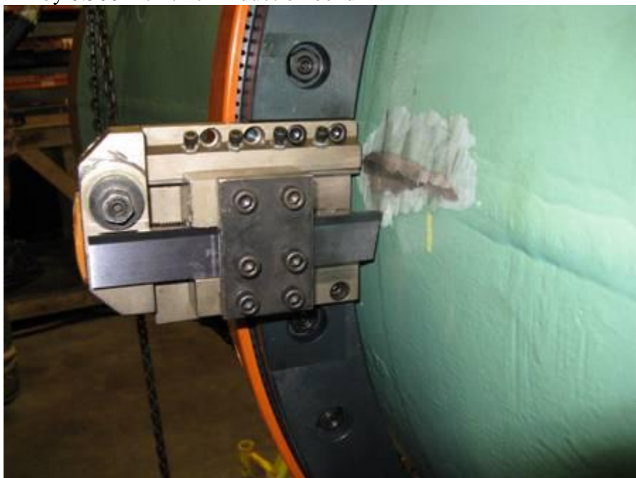
Figure 50. Cutting blade attachment and ground longitudinal seam weld
