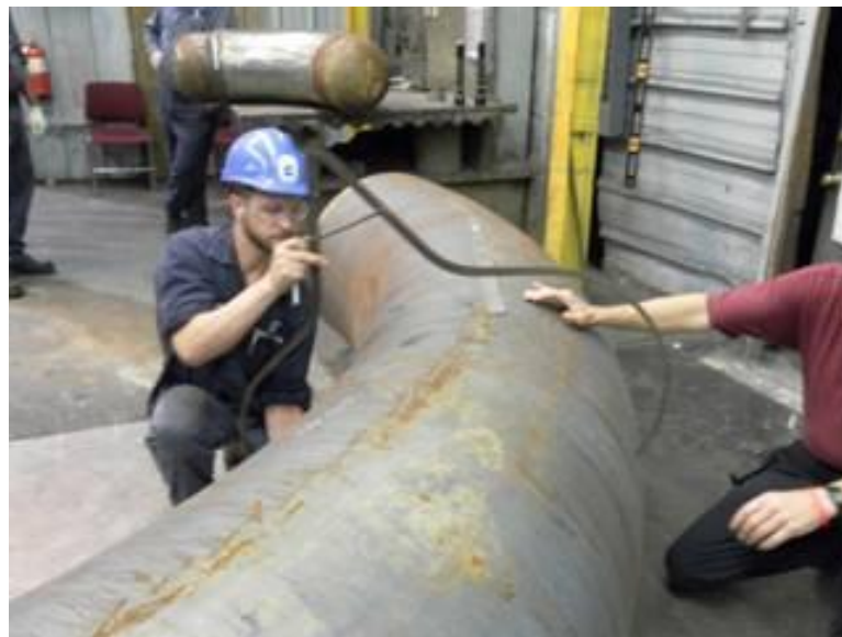
Figure 12. Dimensional check of diameter and out-of-roundness
