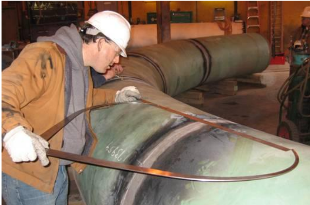
Figure 28. OD measurement using calipers – Part 2
