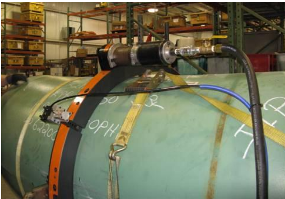
Figure 48. Pneumatic motor of Steel Split Frame® equipment
