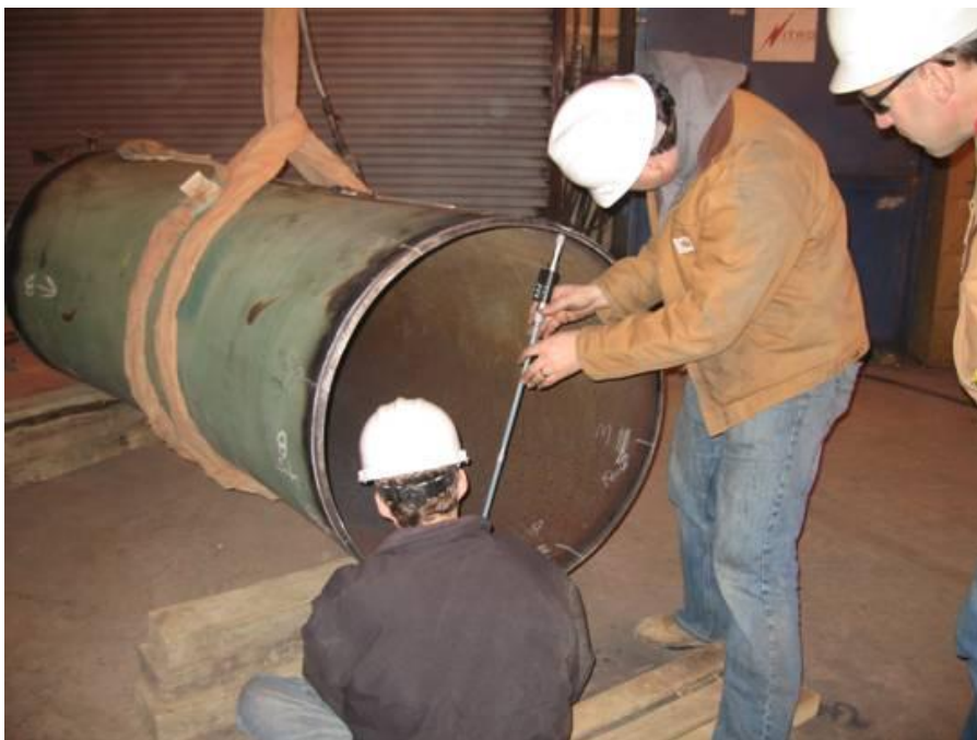
Figure 32. ID measurement using micrometer
