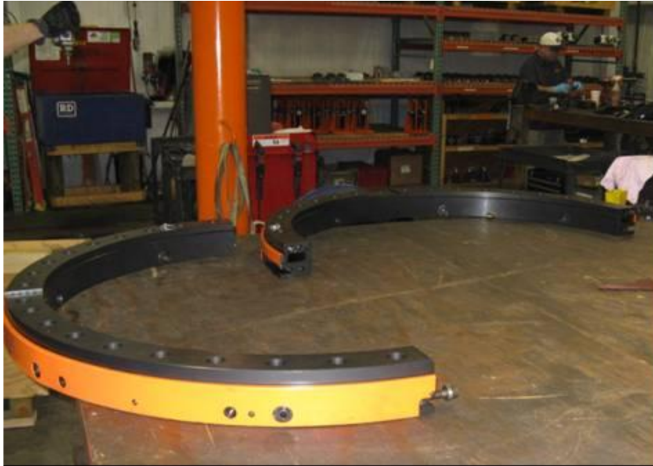
Figure 47. Body of Steel Split Frame® equipment showing split clamshell design
