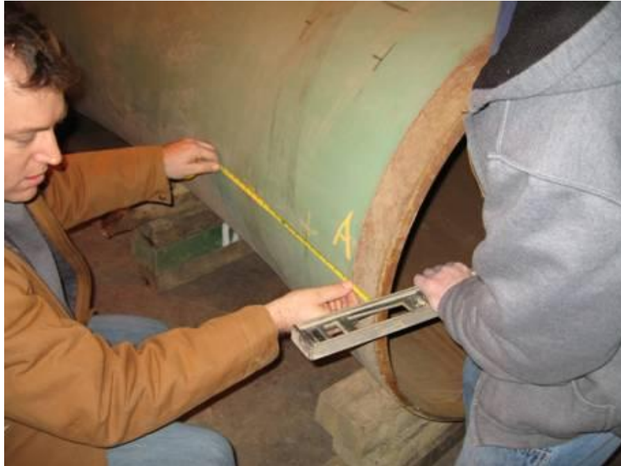
Figure 24. Determining location of true tangent
