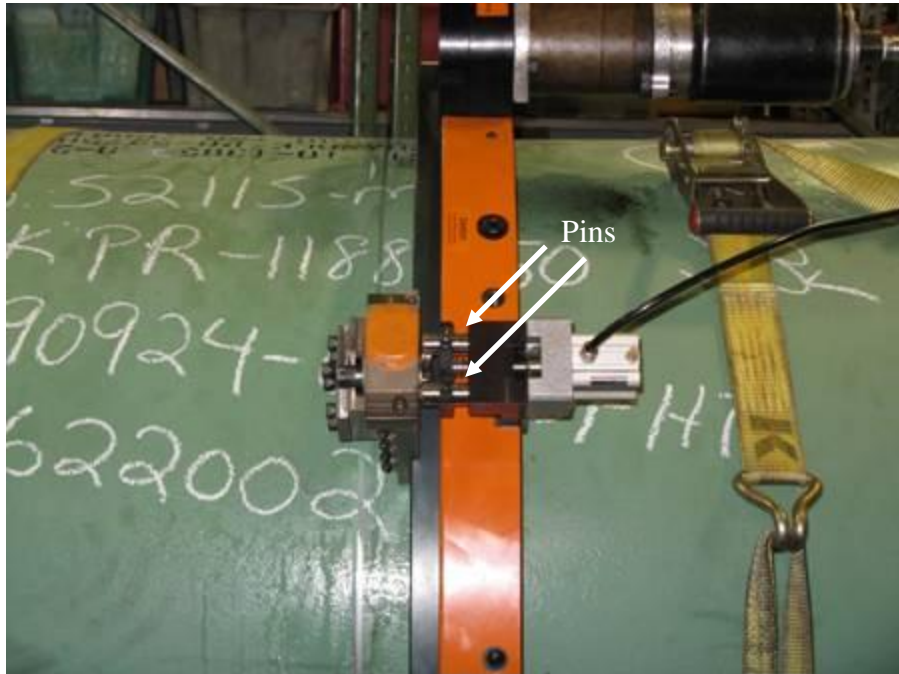
Figure 53. Controller pins engaging cutting blade
