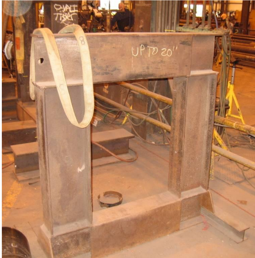
Figure 81. Load frame used for factory re-rounding of elbows
