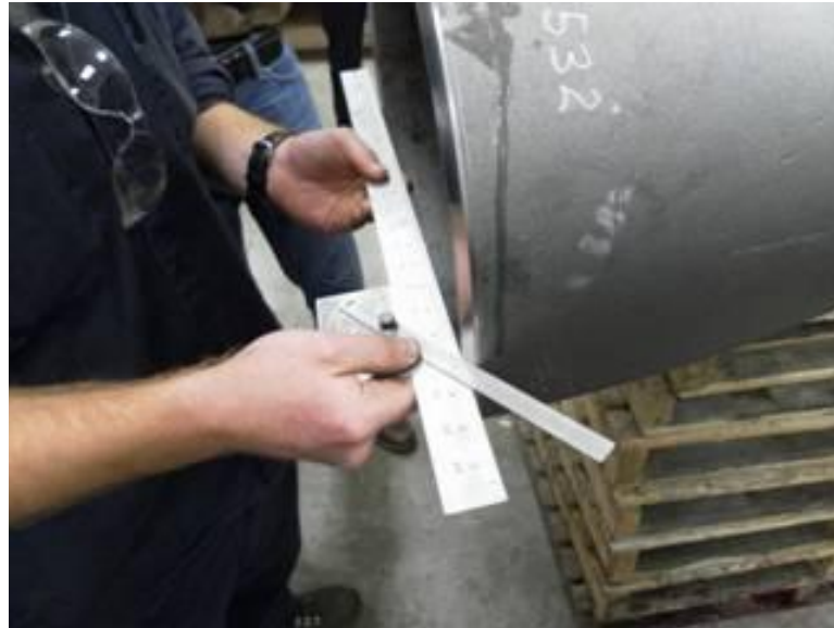
Figure 11. Dimensional check of end preparations
