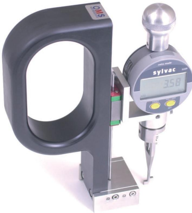
Figure 80. More-sophisticated device for measuring internal misalignment
