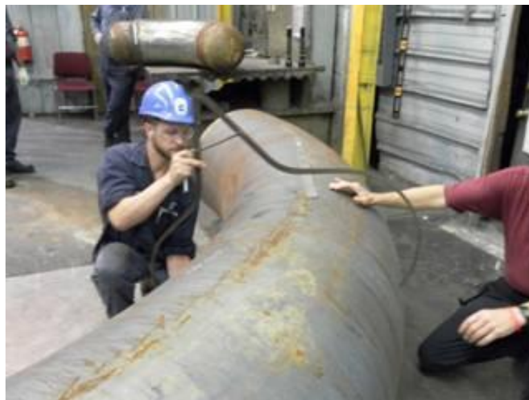
Figure 12. DIMENSIONAL CHECK OF DIAMETER AND OUT-OF-ROUNDNESS
