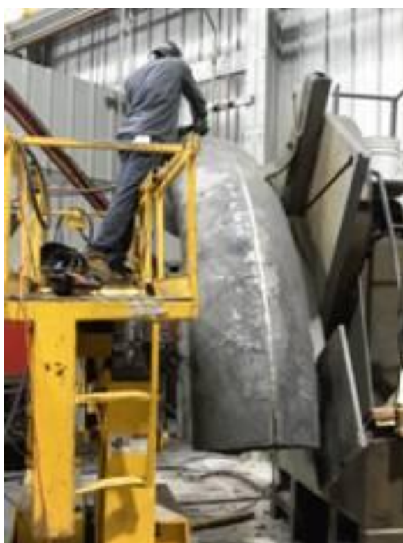
Figure 8. SEAM WELDING USING SUBMERGED ARC WELDING
