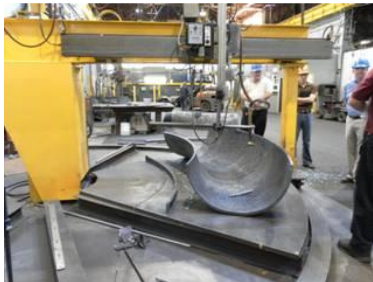
Figure 6. TRIMMING OF ELBOW HALVES
