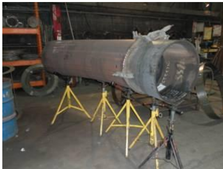
Figure 4. PIPE PUP SECTION BEING ATTACHED TO FACTORY-SEGMENTED INDUCTION BEND
