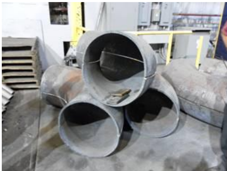
Figure 7. ASSEMBLY OF ELBOW HALVES
