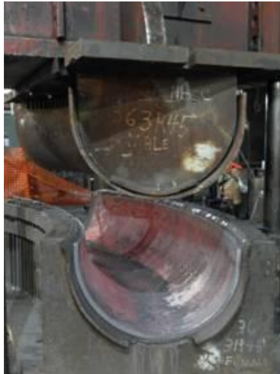
Figure 5. HOT FORMING OF ELBOW HALVES
