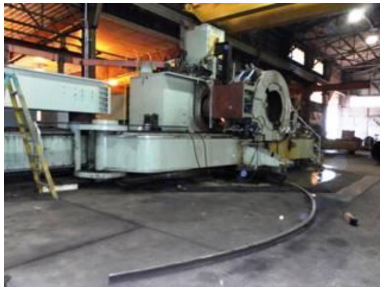
Figure 2. INDUCTION BENDING MACHINE
