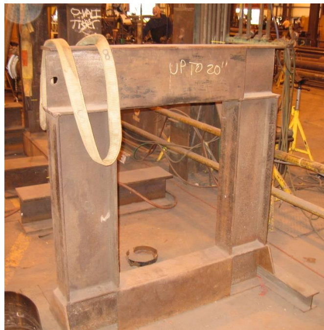
Figure 14. LOAD FRAME USED FOR RE-ROUNDING ELBOWS
