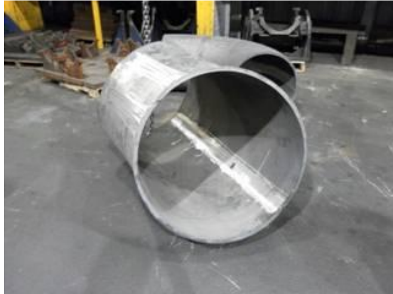
Figure 9. GRINDING OF LONGITUDINAL SEAM WELDS
