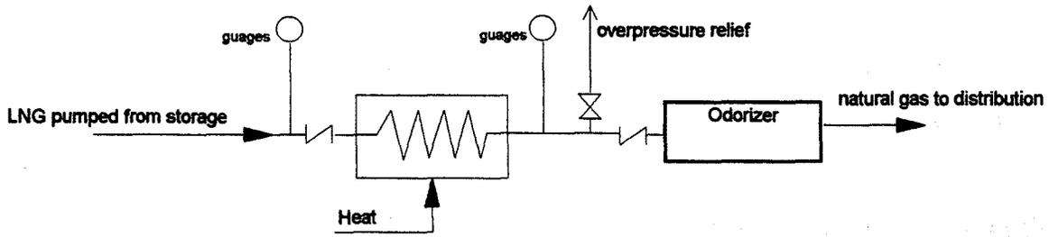
contacted with an intermediate fluid, such as an Ethylene Glycol-water solution, which is pumped through the heat exchanger after being heated by combustion gases. The most commonly used vaporizer in the U.S. is the Direct Fired type. Both types of vaporizers utilize propane or other liquid that does not freeze at LNG temperatures.
