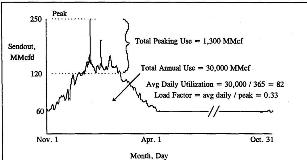
For this particular LDC, without some sort of peakshaving capability, a pipeline capacity of 250 MMcfd would have to be reserved to transport supplies to serve the peak day. This arrangement results in a load factor of 0.33, and corresponding unit cost of pipeline service, calculated as
